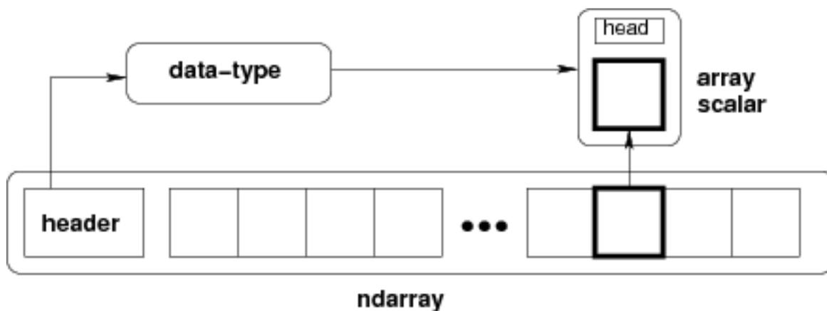
Fig. 1: **Figure** Conceptual diagram showing the relationship between the three fundamental objects used to describe the data in an array: 1) the *ndarray* itself, 2) the *data-type* object that describes the layout of a single fixed-size element of the array, 3) the *array-scalar* Python object that is returned when a single element of the array is accessed.
