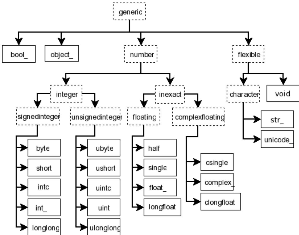
Fig. 2: **Figure:** Hierarchy of type objects representing the array data types. Not shown are the two integer types `intp` and `uintp` which just point to the integer type that holds a pointer for the platform. All the number types can be obtained using bit-width names as well.
