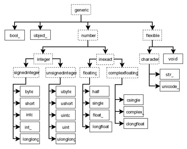
Fig. 2: **Figure:** Hierarchy of type objects representing the array data types. Not shown are the two integer types intp and uintp which just point to the integer type that holds a pointer for the platform. All the number types can be obtained using bit-width names as well.
