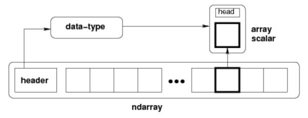
Fig. 1: **Figure** Conceptual diagram showing the relationship between the three fundamental objects used to describe the data in an array: 1) the ndarray itself, 2) the data-type object that describes the layout of a single fixed-size element of the array, 3) the array-scalar Python object that is returned when a single element of the array is accessed.
