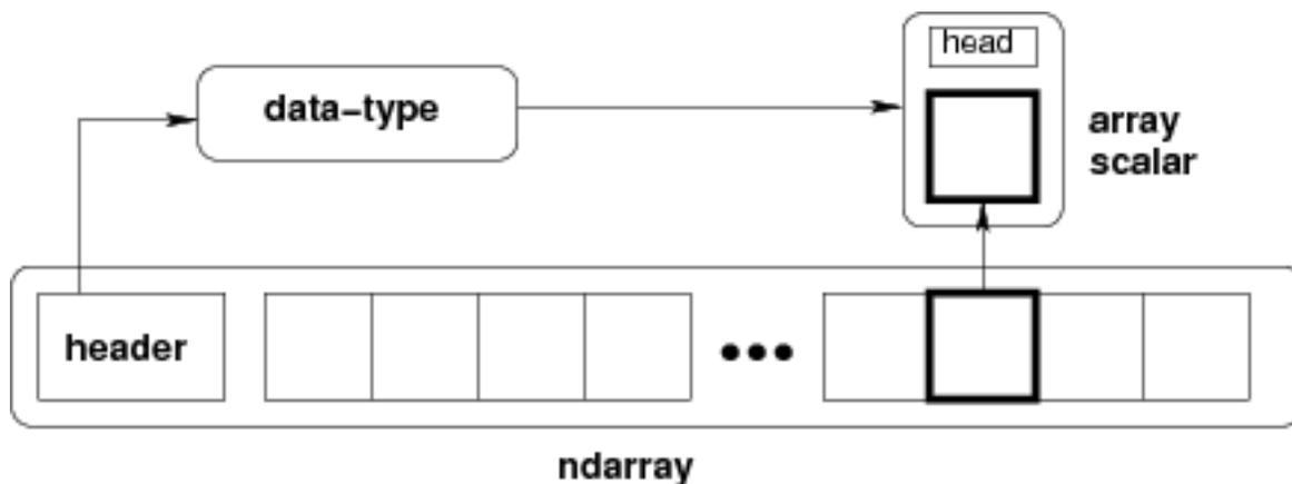
Figure 1.1: **Figure** Conceptual diagram showing the relationship between the three fundamental objects used to describe the data in an array: 1) the *ndarray* itself, 2) the *data-type object* that describes the layout of a single fixed-size element of the array, 3) the *array-scalar Python object* that is returned when a single element of the array is accessed.
