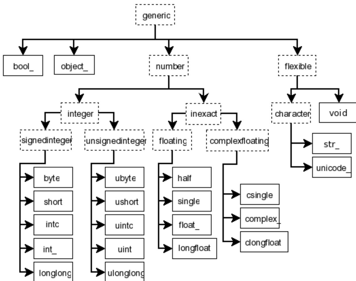
Figure 1.2: **Figure:** Hierarchy of type objects representing the array data types. Not shown are the two integer types `intp` and `uintp` which just point to the integer type that holds a pointer for the platform. All the number types can be obtained using bit-width names as well.
